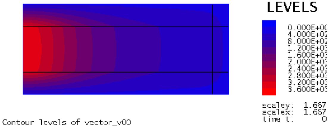
Figure 1. Temperature distribution in laser heated diamond cell from finite element calculations. The sample radius is 90 microns and the thickness is 40 microns. The laser beam is Gaussian with power of 19 Watts. The insulation medium is argon.
