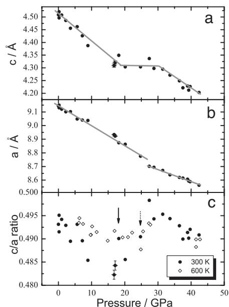
**Fig. 4.** Lattice parameters of  $\text{Fe}_3\text{S}$  versus pressure at 300 and 600 K. (a) Lattice parameter  $c$  versus pressure at 300 K. (b) Lattice parameter  $a$  versus pressure at 300 K. (c)  $c/a$  ratio versus pressure at 300 and 600 K. For clarity, the  $c$  and  $a$  data at 600 K are not shown. The solid arrow indicates the valley in the 300 K data. The dotted arrow indicates the valley in the 600 K data. The error bars are estimated from multiple x-ray measurements.
